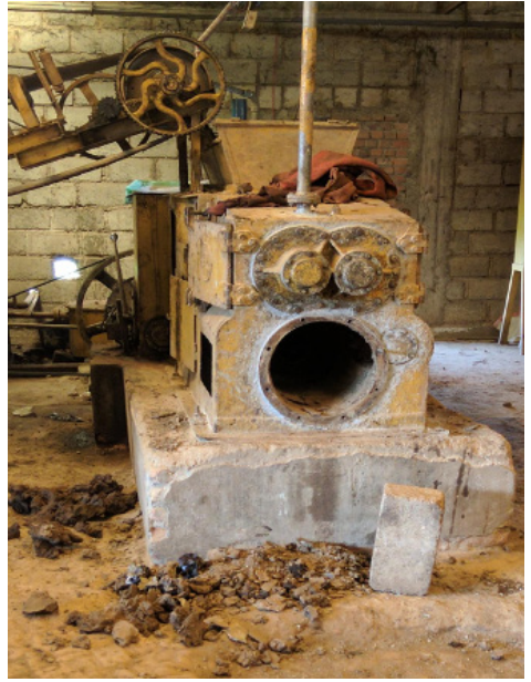
Damaged clay extruder in need of repair
