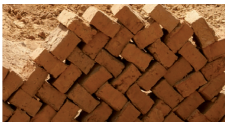
Well aerated storage until adobes complete drying
